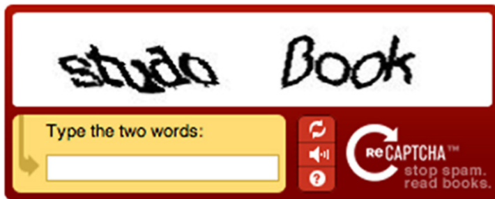
Figure 3: A typical CAPTCHA can help turn back a layer 7 attack.
